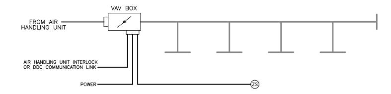
Cooling only VAV box served by an upstream air handling unit. The VAV box serves a single zone with a zone sensor in the zone. Air handling unit interlock and/or DDC communication link varies with the application.
