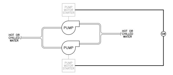
Pumping system for hot or chilled water applications. One pump or both pumps run, depending upon the application and how the pumps are sized. Pump motors are either three phase or single phase. Refer to starter sheet for starter descriptions, selections, and pricing. If pump motors are single phase, then delete the starters.
