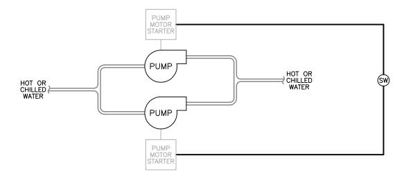
Pumping system for hot or chilled water applications. One pump or both pumps run, depending upon the application and how the pumps are sized. Pump motors are either three phase or single phase. Refer to starter sheet for starter descriptions, selections, and pricing. If pump motors are single phase, then delete the starters.
