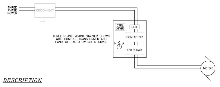
Three phase motor starter consisting of a coil/contactor and a solid state overload block, housed in a general purpose NEMA 1 or weatherproof NEMA 3R enclosure. Options include control transformer, selector switch or start/stop pushbuttons, pilot lights, and auxiliary contacts.
