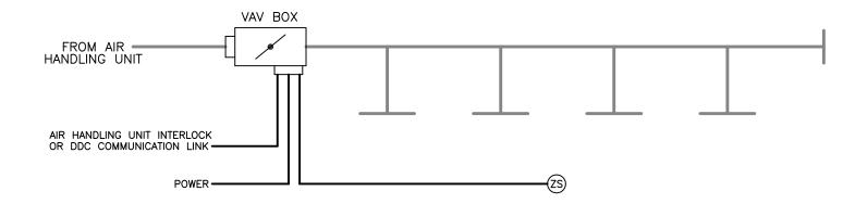
Cooling only VAV box served by an upstream air handling unit. The VAV box serves a single zone with a zone sensor in the zone. Air handling unit interlock and/or DDC communication link varies with the application.
