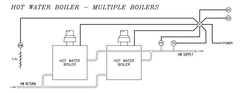
Multiple hot water boilers (single or dual stage) serving a common hot water system. The hot water temperature is controlled by firing the required number of boiler stages. Control is either straight temperature control, or reset control based on outside air temperature. Boiler control with the controller selected here is limited to four stages (two dual stage boilers, or up to four single stage boilers).
